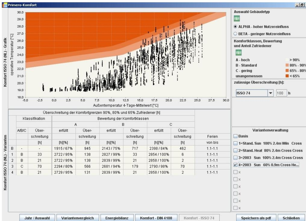
Figure 4 Evaluation of comfort by ISSO 74 (2004) for a simulated summer period. Every point corresponds to one hour of the period of use. The Comfort classes A, B and C are marked in different red colours (Primero-Comfort screenshot).
