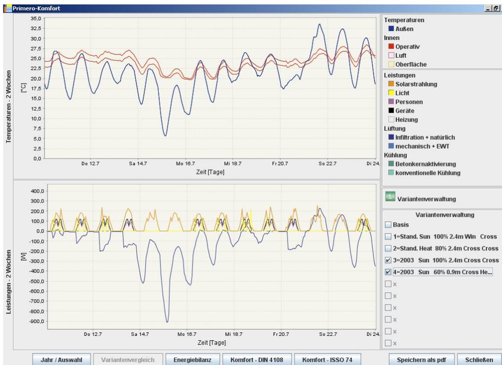
Figure 6 Comparison of operative temperature and energy fluxes for 2 different control strategies for artificial light (reference point in 2.4 / 0.9m depth), hot summer weather (2003). Note that for reference point 0.9m there is in the whole period of 14 days no artificial light contrary reference point 2.4m (yellow lines), this is the reason for the different operative temperatures! (Primero-Comfort screenshot).
