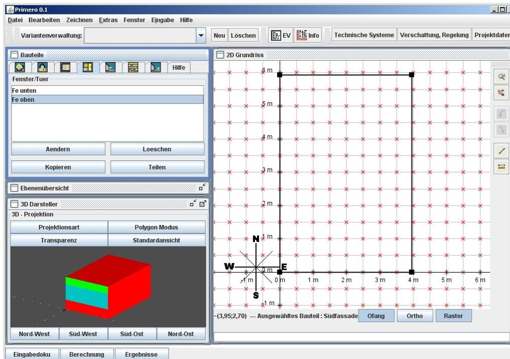
Figure 2 Reference room with two windows with different control strategy of shading (lower part cut off, upper part horizontal), main user interface of Primero-Comfort.
