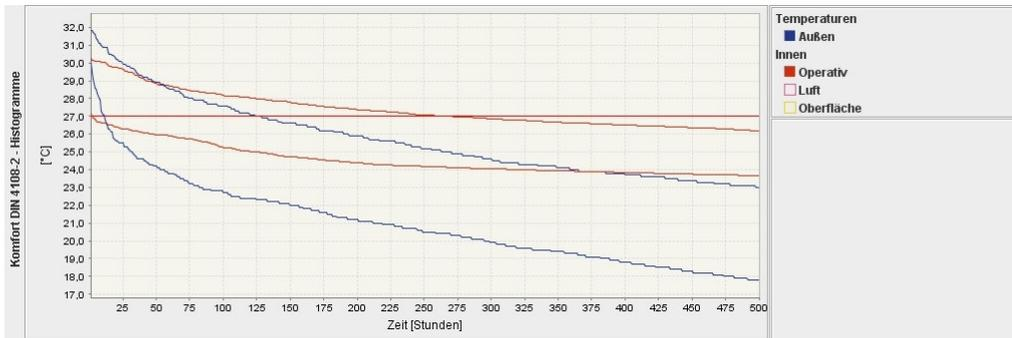
Figure 5 Histogram (number of hours with temperature above a certain value) of temperatures outside (blue lines) and resulting operative temperature inside for the same room (red lines), (Primero-Comfort screenshot).
